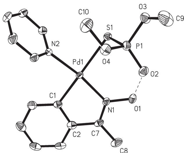
**Fig. 3** Structure of complex **3** in the crystal. Selected bond lengths (Å) and angles (°). Pd(1)–C(1) 1.995(3), Pd(1)–N(1) 2.017(3), Pd(1)–N(2) 2.038(3), Pd(1)–S(1) 2.4609(10), S(1)–P(1) 1.982(1); C(1)–Pd(1)–N(1) 79.88(12), C(1)–Pd(1)–N(2) 93.62(12), N(1)–Pd(1)–N(2) 170.58(11), C(1)–Pd(1)–S(1) 172.81(9), N(1)–Pd(1)–S(1) 99.54(8), N(2)–Pd(1)–S(1) 87.76(8), P(1)–S(1)–Pd(1) 96.46(5).
