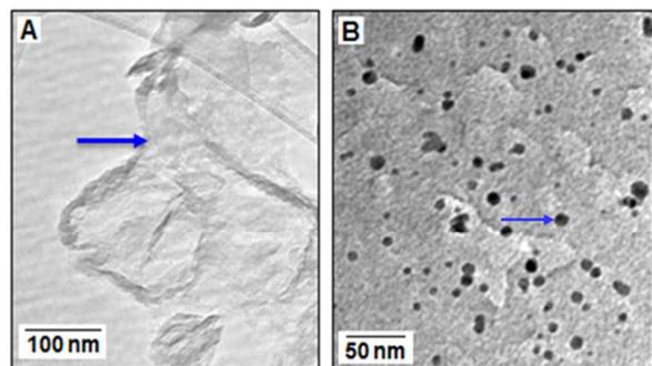
Figure 1: TEM image of the carbon nitride and carbon nitride supported palladium nanoparticles (indicated by the arrows).
