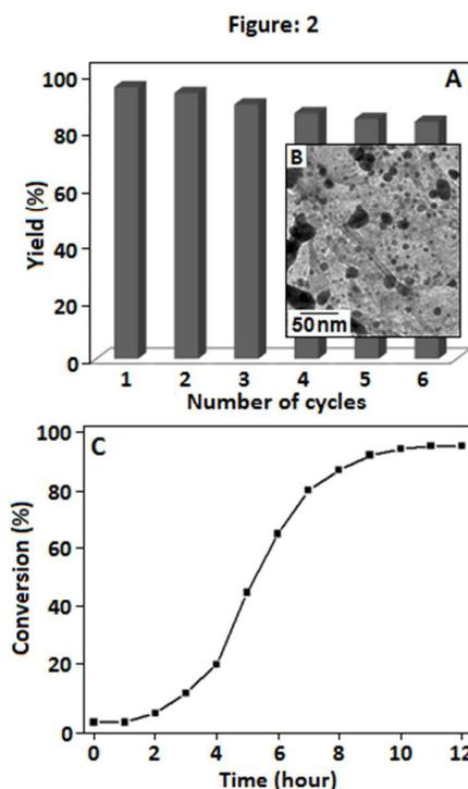
**Figure 2:** (A) The histogram from the recyclability study of the Pd-CN catalyst system. (B) The TEM image of the used catalyst (Pd-CN), at the end of the sixth cycle. (C) The graphical representation of the kinetic study for the aryl-amine coupling reaction as a function of time.
