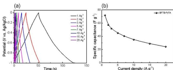
**Fig. 5.** (a) GCD curve of the BFTB-PyTA electrode measured at various current densities ( $\text{A g}^{-1}$ ). (b) Calculated specific capacitances of the BFTB-PyTA electrode at various current densities.
