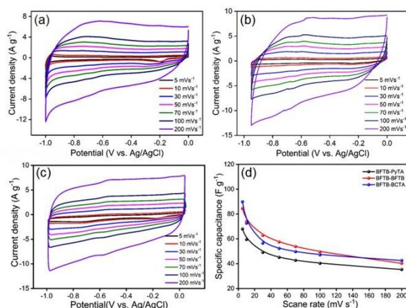
**Fig. 4** (a–c) CV curves of the (a) BFTB-PyTA, (b) BFTB-BFTB, and (c) BFTB-BCTA electrodes measured at various scan rates ( $\text{mV s}^{-1}$ ). (d) Gravimetric specific capacitance of the BFTB-PyTA, BFTB-BFTB and BFTB-BCTA electrodes at various scan rates.
