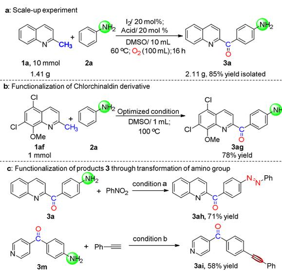
**Scheme 2** Demonstration of synthetic value of this new reaction. Condition a: **3a** (3 equiv.), PhNO<sub>2</sub> (0.5 mmol), KOH (5 equiv.), DMF (3 mL), 150 °C, 24 h. Condition b: **3m** (1.3 equiv.), phenylacetylene (0.4 mmol), Pd(OAc)<sub>2</sub> (5 mol%), tri(furan-2-yl)phosphane (15 mol%), *t*-BuONO (1.3 equiv.), AcOH (1.3 equiv.), DMSO (1 mL), 35 °C, N<sub>2</sub>, 16 h.
