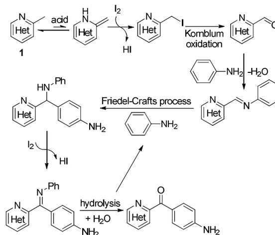
Scheme 3 Proposed mechanism for the metal-free oxidative acylation.
