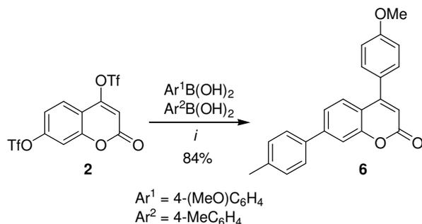
**Scheme 4.** Synthesis of **6**. Conditions: i, 1) **2** (1.0 equiv.), 4-(MeO)C<sub>6</sub>H<sub>4</sub>B(OH)<sub>2</sub> (1.0 equiv.), Pd(PPh<sub>3</sub>)<sub>4</sub> (3 mol %), K<sub>2</sub>CO<sub>3</sub> (2M), toluene, 65 °C, 6 h; 2) (4-MeC<sub>6</sub>H<sub>4</sub>)B(OH)<sub>2</sub> (1.2 equiv.), Pd(PPh<sub>3</sub>)<sub>4</sub> (6 mol %), K<sub>2</sub>CO<sub>3</sub> (2M), dioxane, 110 °C, 6 h.
