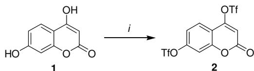
**Scheme 1.** Synthesis of **2**, Conditions: *i*, **1** (1.0 equiv.), pyridine (4.0 equiv.), CH<sub>2</sub>Cl<sub>2</sub>, Tf<sub>2</sub>O (2.4 equiv.), 50 °C, 4 h.
