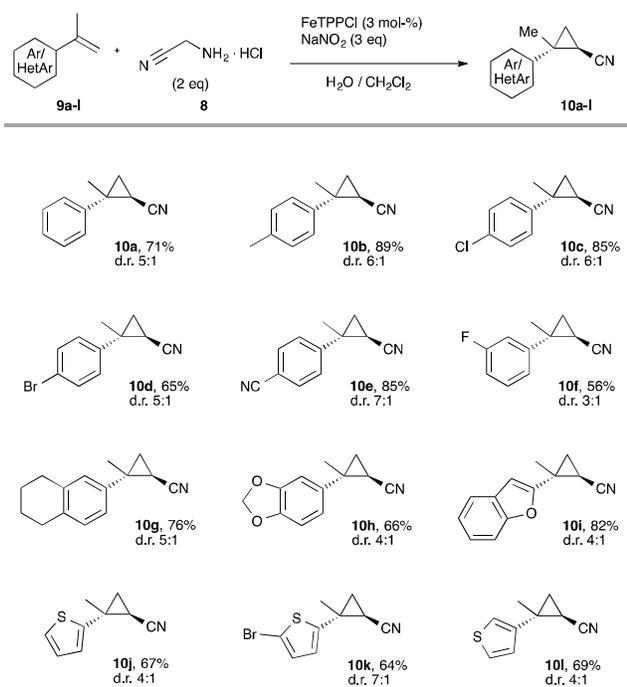
**reaction conditions:** 0.4 mmol styrene (**9a-l**), 3 mol-% FeTPPCL, 2 eq aminoacetonitrile hydrochloride were dissolved in  $\text{H}_2\text{O}/\text{CH}_2\text{Cl}_2$  (1 mL / 100  $\mu\text{L}$ ).  $\text{NaNO}_2$  (3 eq) dissolved in 1 mL water was added over a period of 10 h at rt; the resulting mixture was stirred for another 4 h at rt; reported yields refer to the *trans* product after column chromatography; the d.r. was determined from the crude reaction mixture by  $^1\text{H-NMR}$ .
