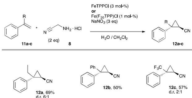
**reaction conditions:** 0.4 mmol styrene (**11a-c**), 3 mol-% FeTPPCL, 2 eq aminoacetonitrile hydrochloride were dissolved in  $\text{H}_2\text{O}/\text{CH}_2\text{Cl}_2$  (1 mL / 100  $\mu\text{L}$ ).  $\text{NaNO}_2$  (3 eq) dissolved in 1 mL water was added over a period of 10 h at rt; the resulting mixture was stirred for another 4 h at rt; reported yields refer to the *trans* product after column chromatography; the d.r. was determined from the crude reaction mixture by  $^1\text{H-NMR}$ .
