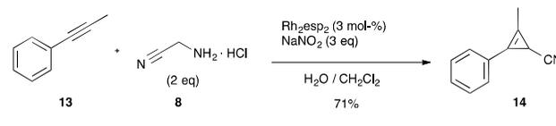
**Scheme 2.** Cyclopropanation reaction with  $\text{Rh}_2\text{esp}_2$ .
