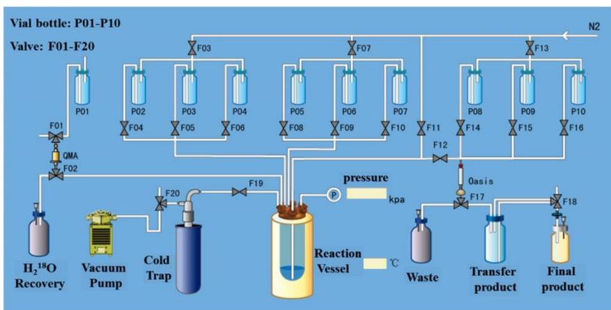
FIGURE 1 Module diagram (BIBD-F) of automated radiosynthesis of [<sup>18</sup>F]AV-45 ([<sup>18</sup>F]5).
