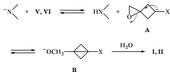
Presumably, the observed isomerization direction (**V, VI** → **I, II**) is governed by the stage including transformation of carbanion **A** into alcoholate ion **B**; the latter is more stable due to high electronegativity of the oxygen atom. Aprotic medium and some excess of a strong base are necessary conditions for the process to be controlled by the transformation **A** → **B** (Scheme 4).
