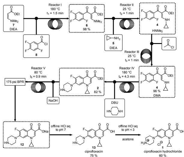
**Scheme 5.** Flow scheme of continuous total synthesis of ciprofloxacin. 1.0 equiv. of **7**, 1.2 equiv. of **8**,<sup>[17]</sup> 1.15 equiv. of DIEA, 1.25 equiv. of **5**, 1.15 equiv. of DIEA, 1.2 equiv. of acetyl chloride, 3.5 equiv. of DBU, 3.5 equiv. of piperazine, 6.0 equiv. of NaOH. See supporting information for details. DBU = 1,8-Diazabicyclo[5.4.0]undec-7-ene.
