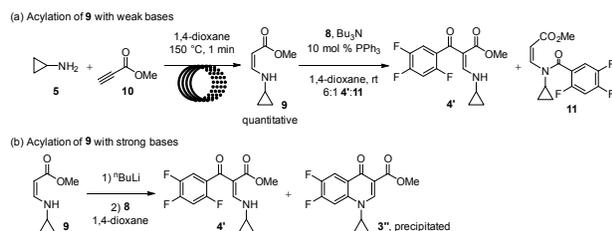
**Scheme 3.** Alternative unoptimized methods for preparation of **4'**. Conditions for preparation of **9** in a continuous flow reactor: 1.0 equiv. of **5** (2.0 M in 1,4-dioxane, 222.0  $\mu$ L/min), 1.0 equiv. of **10** (2.0 M in 1,4-dioxane, 222.0  $\mu$ L/min), 150  $^{\circ}$ C, 1 min, 200 psi back pressure.
