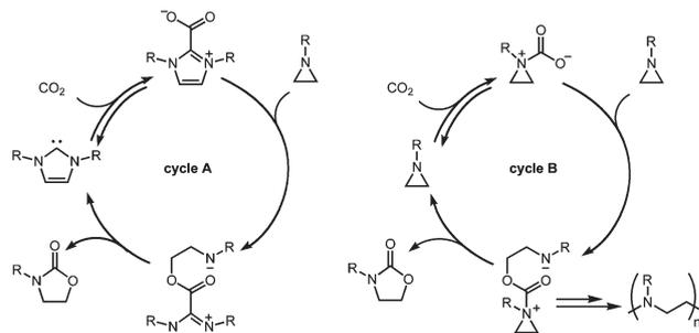
**Fig. 3** Possible mechanisms of cycloaddition of tertiary aziridines with CO<sub>2</sub>.
