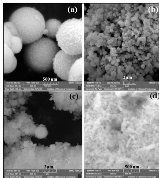
**Fig. 4** SEM images of Cu NPs by changing the metal precursor (a) and (b)  $Cu_2O$  NPs from  $Cu(NO_3)_2$  (c) and (d)  $Cu(OH)_2$  microparticles synthesised from  $CuCl_2$ .
