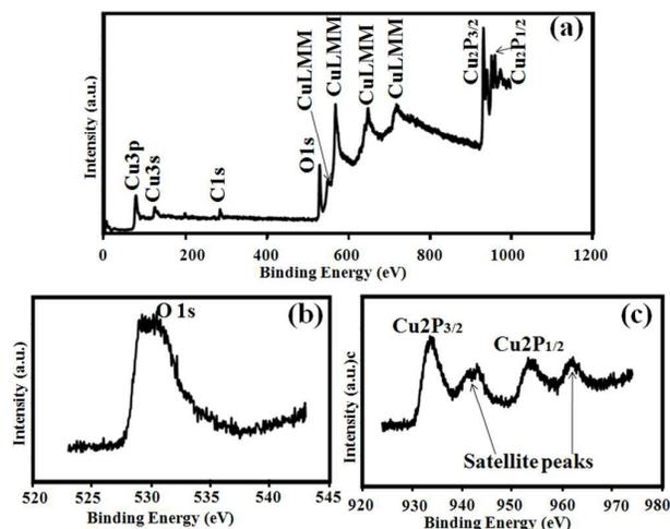
**Fig. 3** XPS spectra of CuO NPs (d): (a) survey spectrum, (b) O1s region and (c) Cu2p region.
