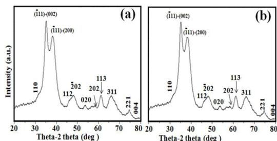
**Fig. 2** XRD pattern of CuO NPs (a) 3:7 and (b) 7:3 of EG/ water as solvent system
