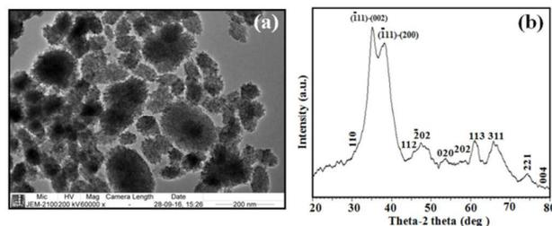
**Fig. 7** (a) TEM and (b) XRD analysis of CuO NPs after recycle.
