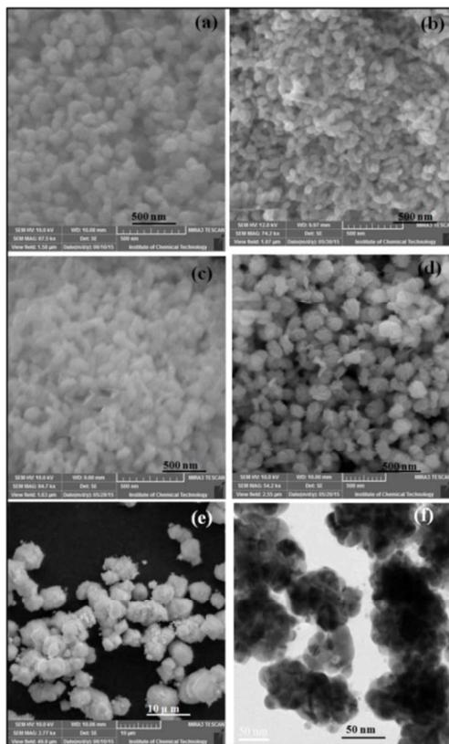
**Fig. 1** FEG-SEM images of CuO NPs synthesized at different volume ratio of EG/water in mL (a) 1:9 (b) 3:7 (c) 5:5 (d) 7:3 (e) 9:1 (f) TEM image of 7:3 of EG/water synthesized at 600 W for 4 min.
