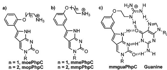
**Figure 2.** Structures of modified PhpCs designed to engage guanine with an additional hydrogen bond. (a) Previously studied moePhpC and newly synthesized mopPhpC; (b) meta-substituted PhpCs mmePhpC ( $n = 1$ ) and mmpPhpC ( $n = 2$ ); (c) proposed interaction of guanidino-PhpC (mmguaPhpC) with guanine.
