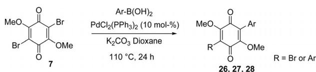
Scheme 11. Mono- and dicoupling by Suzuki–Miyaura reactions on dibromo intermediate **7**.
