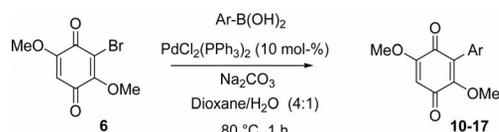
Scheme 6. Synthesis of the first generation of embelin derivatives through Suzuki–Miyaura coupling reactions using automated parallel synthesizer.
