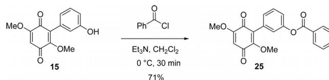
Scheme 10. Esterification reaction to prepare benzoquinone **25**.
