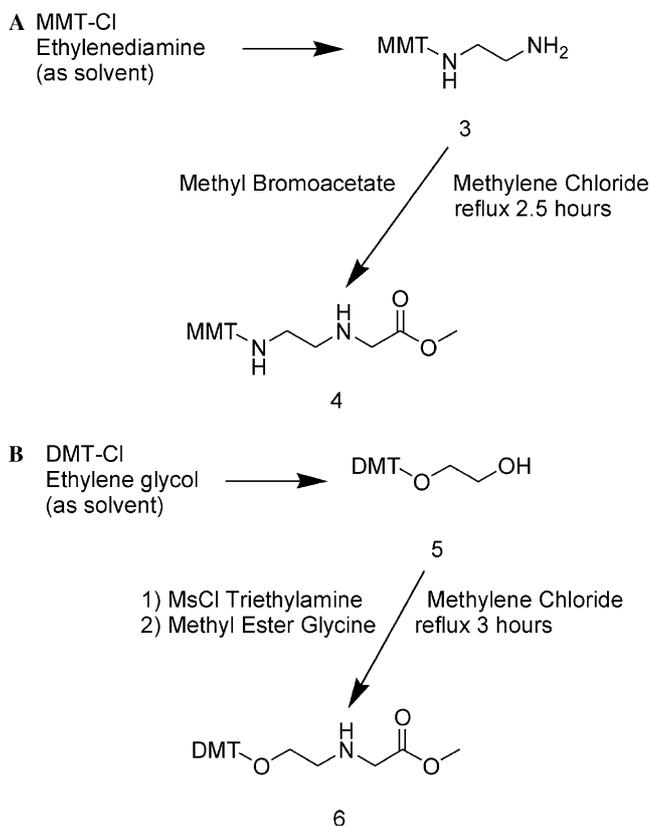
**Scheme 1.** (A) MMT-protected aminoethyl PNA glycine backbone synthesis. (B) DMT-protected hydroxyl ethyl PNA–DNA linker backbone synthesis.
