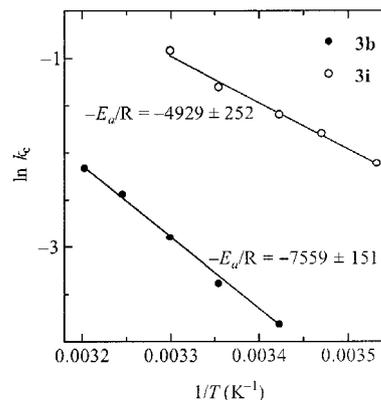
Figure 7.  $\ln k_c$  vs.  $1/T$  for the 2-(benzoylamino)thiobenzamides **3b** and **3i**
