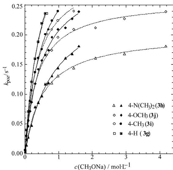
Figure 3. Observed rate constant of the cyclisation ( $k_{\text{obs}}/\text{s}^{-1}$ ) of the 2-[(benzoyl)(methyl)amino]thiobenzamides **3g–j** vs. the concentration  $c$  (solid symbols and solid lines) and vs. the apparent concentration  $c'$  (open symbols and dashed lines) of sodium methoxide ( $c/\text{mol}\cdot\text{L}^{-1}$ ) calculated by means of the  $H_{\text{M}}$  function and Equation (5) at 25 °C
