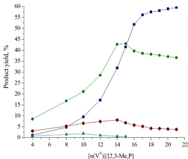
**Fig. 8.** Product distribution dependence on molar  $[n_{V^V}]/[Su]$  ratio in the presence of 0.20 M H<sub>7</sub>PMo<sub>8</sub>V<sub>4</sub>O<sub>40</sub> (HPA-4) solution. Reaction conditions: catalyst ( $c_{V^V} = 0.77 \text{ mol L}^{-1}$ ), 2,3-Me<sub>2</sub>P 0.099 g, atm. N<sub>2</sub>, temperature 50 °C, benzene, organic solvent volume 0.75· $V_{kat}$ . Products: ● – DPQ, ■ – 2,3-Me<sub>2</sub>BQ, ◆ – PPO, ▲ – PP.
