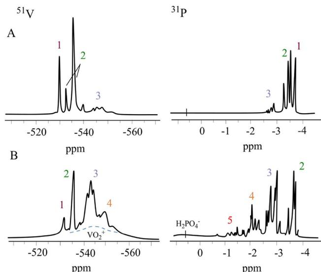
Fig. 3. <sup>31</sup>P and <sup>51</sup>V NMR spectra of aqueous Keggin-type HPA-x solutions: (A) 0.40 M HPA-2 and (B) 0.20 M HPA-4. The numbers 1–5 correspond to individual HP-anions with x of 1–5.
