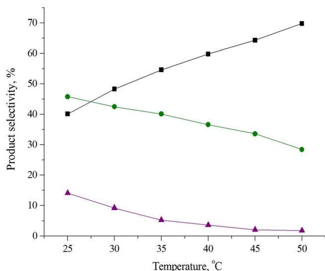
Fig. 7. Product selectivity dependence on reaction temperature in the presence of 0.25 H<sub>13</sub>P<sub>3</sub>Mo<sub>15</sub>V<sub>6</sub>O<sub>74</sub> (HPA-6') solution: (■) – 2,3-Me<sub>2</sub>BQ, (●) – DPQ, (▲) – PPO. Reaction conditions: catalyst 7.5 mL ( $n_{V^V} = 1.07 \cdot 10^{-2}$  mol), 2,3-Me<sub>2</sub>P 0.066 g, air atmosphere, benzene 5.5 mL, molar  $[n_{V^V}]/[2,3\text{-Me}_2\text{P}]$  ratio 20. Substrate conversion is 100%.
