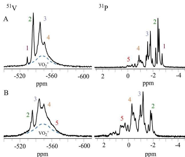
Fig. 4. <sup>31</sup>P and <sup>51</sup>V NMR spectra of aqueous modified-type HPA-x' solutions: (A) 0.25 M HPA-7' and (B) 0.25 M HPA-10'. The numbers 1–5 correspond to individual HP-anions with x of 1–5.
