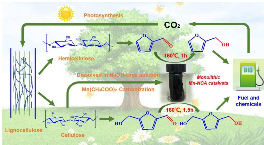
Cellulose-derived monolithic hierarchically porous  $\text{MnO}_x/\text{N}$ -doped carbon aerogel exhibited excellent catalytic activity for upgrading of lignocellulose-derived aldehydes
