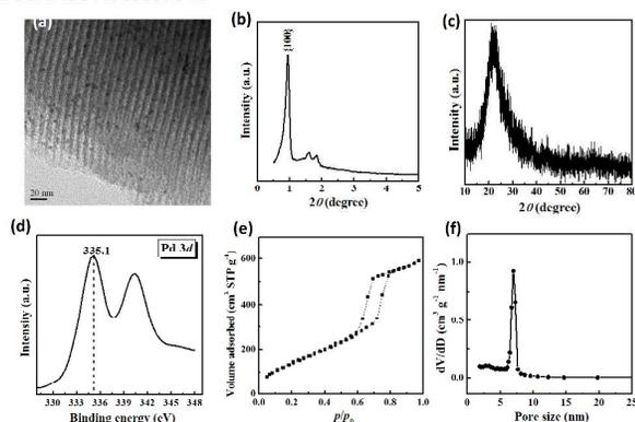
**Fig. 1** (a) TEM image, (b) low-angle XRD pattern, (c) wide-angle XRD pattern, (d) XPS spectrum, (e)  $N_2$  adsorption-desorption isotherms, and (f) pore size distribution of Pd/SBA-15.
