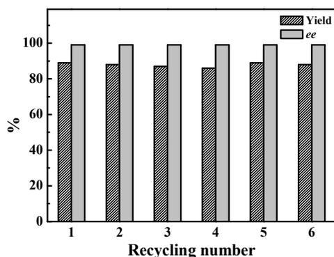
**Fig. 2** Recycling test of the enzyme and Pd@SBA-15 catalysts for microwave-assisted one-pot DKR of *rac*-1-phenylethanol. Reaction conditions: a catalyst containing 2 mg of Pd, 100 mg of Novozym<sup>®</sup> 435, 0.5 mmol of *rac*-1-phenylethanol, 1.5 mmol of vinyl acetate,  $T = 70\text{ }^{\circ}\text{C}$ ,  $P_{\text{H}_2} = 0.03\text{ MPa}$ , 4 mL of *n*-hexane. Each run was conducted for 4 h in recycling test.
