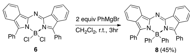
Scheme 5 Synthesis of diphenylboryl benzannulated aza-BODIPY 8 via Cl-aza-BODIPY 6 .
