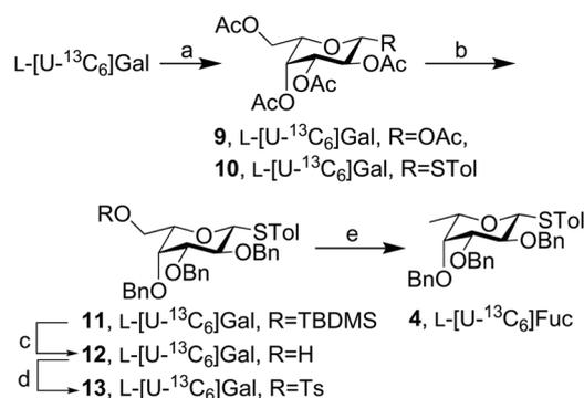
**Scheme 2** Reagents and conditions: (a) 1. NaOAc, Ac<sub>2</sub>O, 140 °C, 30 min, 99% (**9**); 2. MePhSH, BF<sub>3</sub>·Et<sub>2</sub>O, CH<sub>2</sub>Cl<sub>2</sub>, rt, 2 h, 98% (**10**); (b) 1. NaOMe, MeOH, rt, 30 min, 99%; 2. TBDMSCl, pyridine, 0 °C to rt, 4 h, 95%; 3. BnBr, NaH, DMF, 0 °C to rt, 2 h, 79% (**11**); (c) Bu<sub>4</sub>NF, THF, rt, 16 h, 96%; (d) TsCl, pyridine, rt, 3 h, 94%; (e) LiAlH<sub>4</sub>, THF, reflux, 61%.
