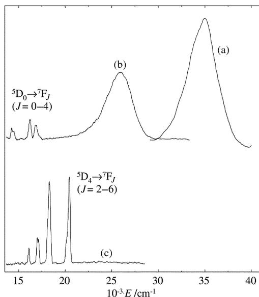
**Fig. 6** Fluorescence (a) and phosphorescence (b) spectra of  $\text{EuL}^2$ , and phosphorescence (c) spectrum of  $\text{TbL}^2$  (solid state, 77 K). The following excitation energies, time delays and bandpaths were used: (a) 42 373  $\text{cm}^{-1}$ , 0  $\mu\text{s}$ , 4 nm; (b) 42 553  $\text{cm}^{-1}$ , 20  $\mu\text{s}$ , 10 nm; (c) 35 714  $\text{cm}^{-1}$ , 20  $\mu\text{s}$ , 2.5 nm.
