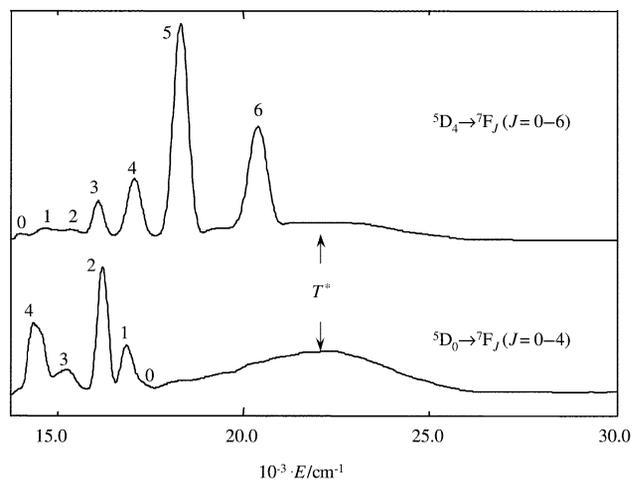
**Fig. 9** Phosphorescence spectra of  $\text{TbL}^4$  (top) and  $\text{EuL}^4$  (bottom),  $5 \times 10^{-5}$  M in  $\text{CH}_3\text{CN}$  at 77 K,  $E_{\text{exc}} = 41\,667\text{ cm}^{-1}$ , time delay = 50  $\mu\text{s}$ , bandpath = 5 nm.
