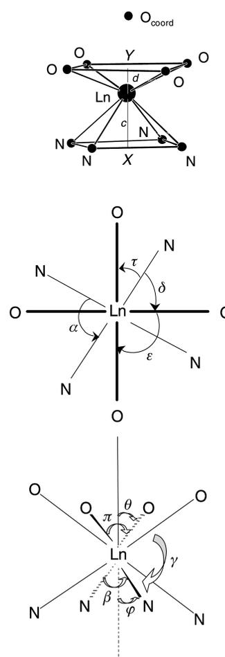
**Fig. 5** Parameters defining a twisted square antiprismatic co-ordination polyhedron: relevant distances, spatial (↗) and projection (↘) angles; *X* and *Y* are the centres of the N<sub>4</sub> and O<sub>4</sub> planes, respectively.
