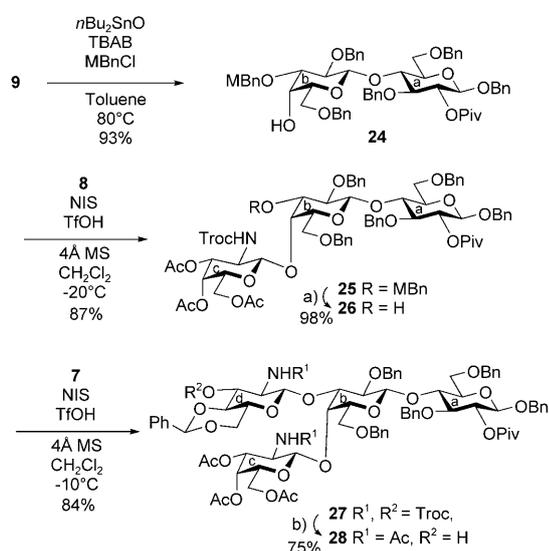
Scheme 7. Synthesis of unit **28** of the glycan part of the target compound. a) TFA/CH<sub>2</sub>Cl<sub>2</sub>, 98%; b) i) Zn, AcOH/MeOH; ii) Ac<sub>2</sub>O/CH<sub>2</sub>Cl<sub>2</sub>-MeOH, 75%. TBAB = *n*-tetrabutylammonium bromide, MBn = *p*-methoxybenzyl, TFA = trifluoroacetic acid.
