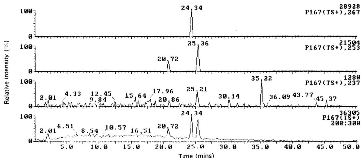
**Figure 4.** HPLC thermospray CAD MS/MS traces obtained for the parents of the *m/z* 167 ion: the peaks at 20.72, 24.34, 25.21 and 25.36 min are candidate metabolites in which the xanthine ring is unchanged. The peak at 35.22 min is the original drug.
