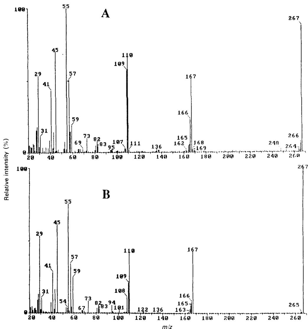
**Figure 9.** CAD MS/MS fragment ion spectra of the chromatographic peak at 24.34 min having  $m/z$  267 as the possible quasi-molecular ion (A) and of synthetic 2,2-dimethyl,3-(1-methylxanthin-7-yl)propionic acid (B).
