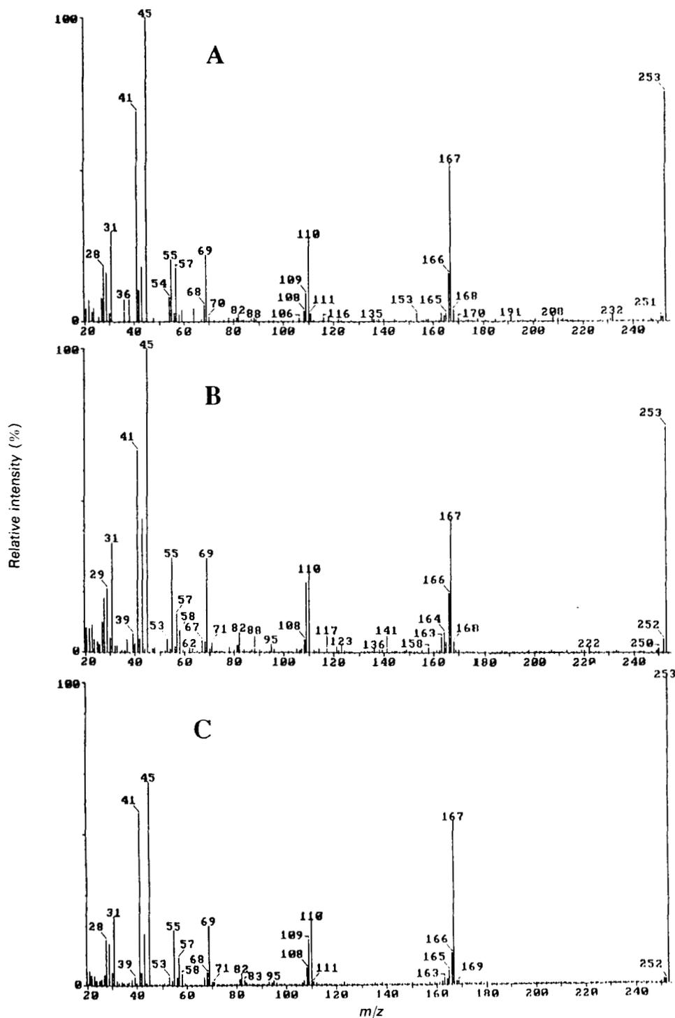
**Figure 8.** CAD MS/MS fragment ion spectra of the two chromatographic peaks having  $m/z$  253 and the possible quasi-molecular ion ((A) peak at 20.72 min and (B) peak at 25.36 min) and of synthetic 1-methyl-7-(2,2-dimethyl-3-hydroxypropyl)xanthine (C).
