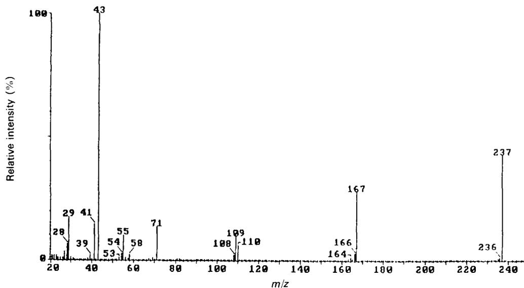
Figure 2. CAD fragment ion spectrum of MX/2/120.
