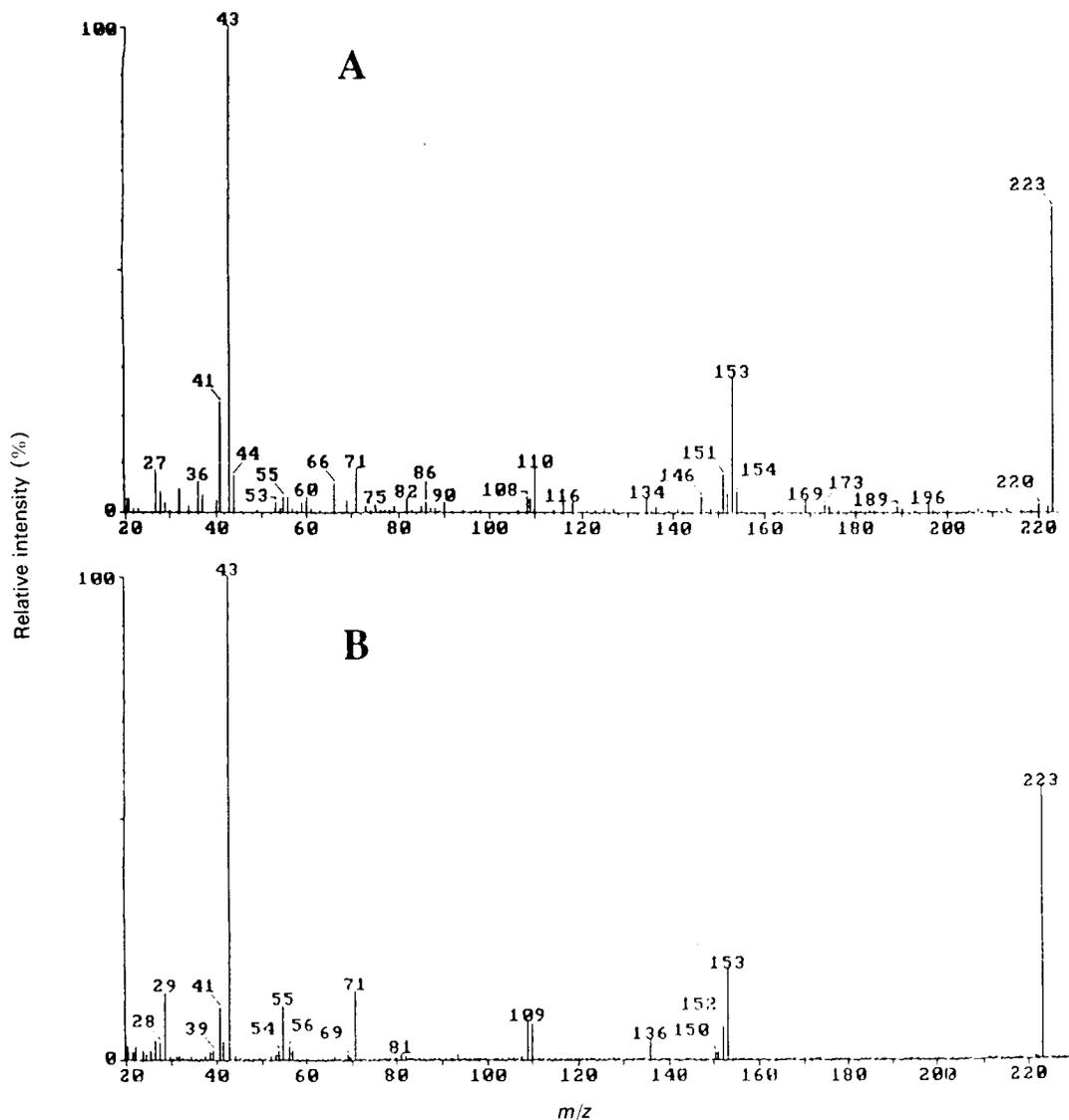
Figure 10. CAD MS/MS fragment ion spectra of the chromatographic peak at 24.34 min having  $m/z$  223 as the possible quasi-molecular ion (A) and of synthetic 7-neopentylxanthine (B).
