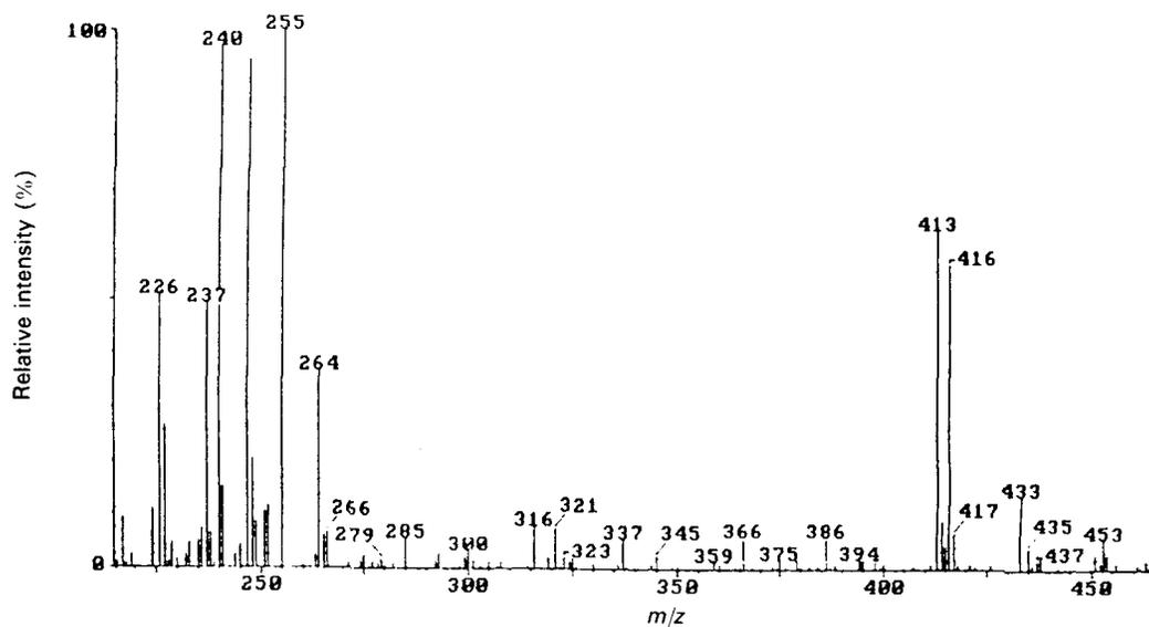
Figure 6. Background-subtracted thermospray mass spectrum of the peak at 25.21 min, obtained from urine of a guinea-pig treated with an equimolar mixture of MX/2/120 and its  $N^1$ -deuterated analogue: the two pairs of peaks at  $m/z$  237 and 240 and  $m/z$  413 and 416 suggest a glucuronide of the unchanged drug.
