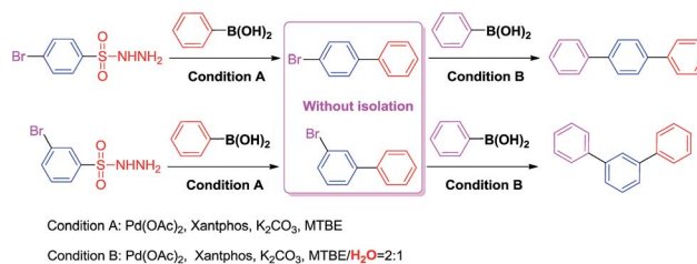
Scheme 2 “One-pot” synthesis of terphenyl.
