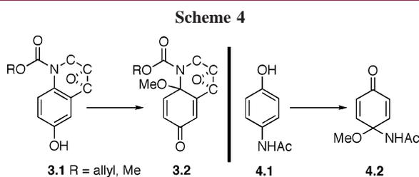
that **4.1** is convertible into **4.2** on treatment with PhI(OAc)<sub>2</sub> (Scheme 4).<sup>9,10</sup> We evaluated a number of nitrogen protecting groups and found that not all of them allow the chemical oxidation **2.1** → **2.2**: *p*-toluenesulfonyl, *t*-butoxycarbonyl,
