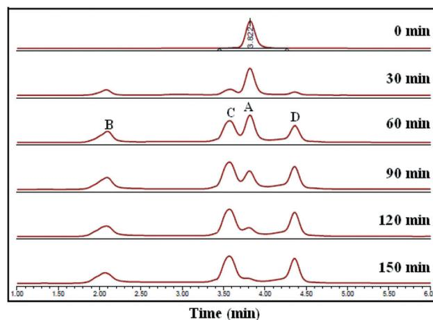
**Fig. 1** HPLC profile for the photolysis of the carbonate **5f** ( $1 \times 10^{-4}$  M) in ACN–H<sub>2</sub>O (50 : 50 v/v) at regular interval of time (0–150 min, time interval = 30 min), (A = **5f**, B = **4f**, C = **1**, D = **1**).**Table 3** Photorelease data of carbonates **5f** in different solvents
