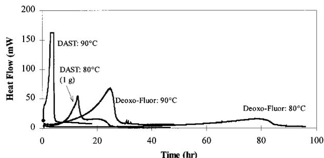
**Figure 1.** Isothermal calorimetry of DAST and Deoxo-Fluor (**1**) reagents.
