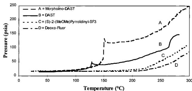
**Figure 2.** Comparison of recorded pressure data from the thermal decomposition of the Deoxo-Fluor (**1**), DAST, and morpholino-DAST reagents in the Radex instrument.
