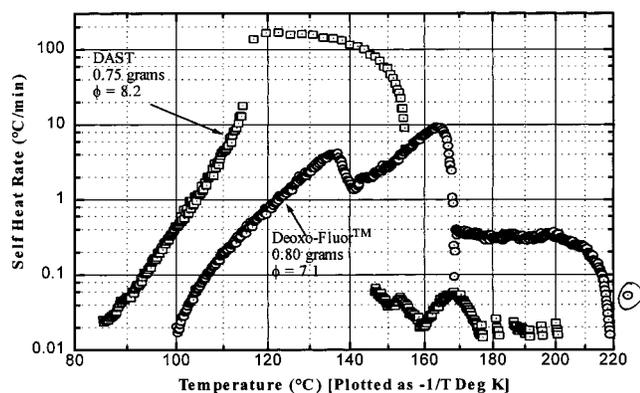
**Figure 3.** Accelerating rate calorimetry of DAST and Deoxo-Fluor reagents.
