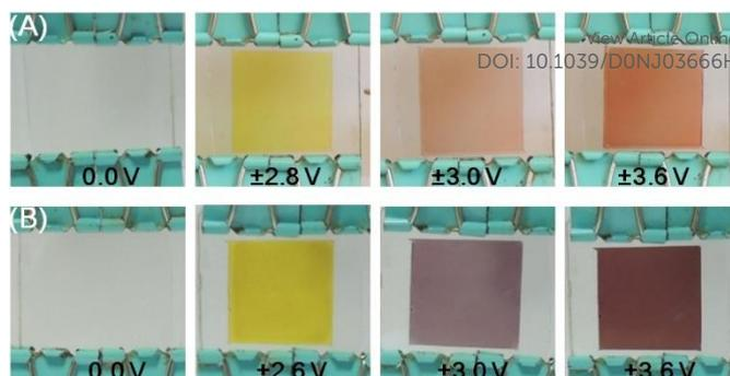
**Fig. 5.** Photograph of the ECDs based on compounds a (A) and f (B) in their bleached (at 0.0 V) and colored states.
