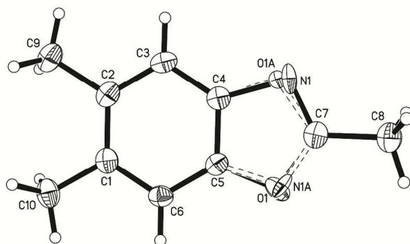
**Figure 1.** ORTEP drawing of 2,5,6-trimethylbenzo[d]oxazole (**2da**, CCDC 1410546) showing 50% probability amplitude displacement ellipsoids. Oxygen and nitrogen atoms are shown disordered as this planar molecule can pack in two different ways occupying practically the same space in the crystalline lattice.
