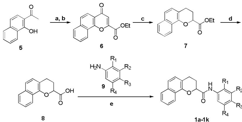
**Scheme 1.** General methods to prepare 1 series. Reagents and conditions: (a) diethyl oxalate, NaOEt, EtOH, reflux, 3 h (b) EtOH, HCl (c) H<sub>2</sub>, 10% Pd/C, EtOH, 24 h (d) KOH, isopropylalcohol/H<sub>2</sub>O, reflux, 3h (after 4 steps yield 50%) (e) CDI, THF, 12 h, 52-75%
