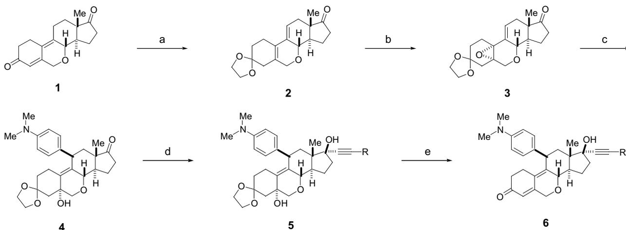
**Scheme 1.** Synthesis of oxa-steroids. Reagents and conditions: (a) (CH<sub>2</sub>OH)<sub>2</sub>, pyridine-HCl, benzene, refluxing, 82%; (b) *m*-CPBA, NaHCO<sub>3</sub>, DCM,  $-30\text{ }^{\circ}\text{C}$ , 70%; (c) Me<sub>2</sub>NC<sub>6</sub>H<sub>4</sub>MgBr, CuCN–2LiCl, THF,  $0\text{ }^{\circ}\text{C}$ , 88%; (d) MeCCMgBr (**6a**, R = Me), THF, rt, 92%; (e) 3 N HCl aq, acetone, 95%.
