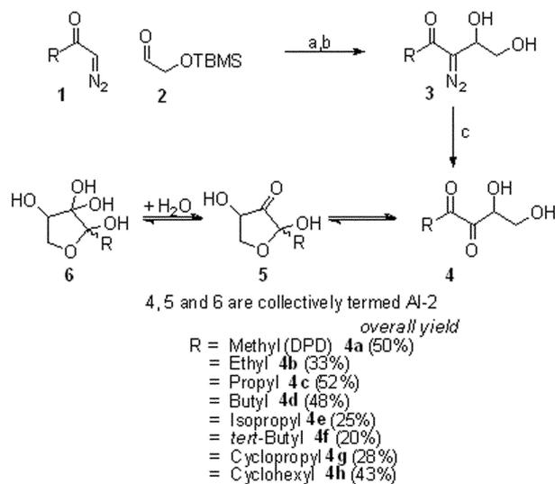
**Scheme 1** A two-pot synthesis of AI-2 and analogues; (a) cat. DBU, MeCN; (b) TBAF (1–3 eq), THF; (c) dimethyl dioxirane; acetone. DBU = 1,8-diazabicyclo[5.4.0]undec-7-ene.
