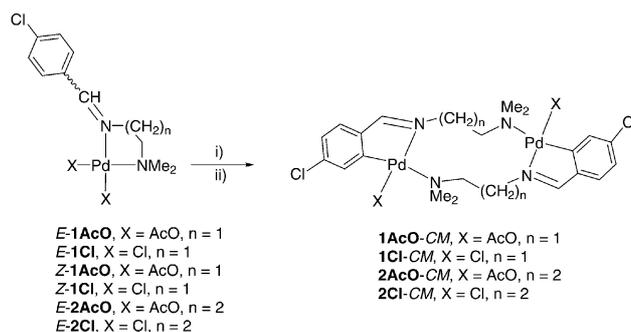
**Scheme 3** Preparation of cyclometallated compounds **1AcO-CM**, **1Cl-CM**, **2AcO-CM** and **2Cl-CM**. Reagents and conditions: (i) AcOH, 60 °C, 5 h; (ii) solvent evaporation and precipitation with diethyl ether.
