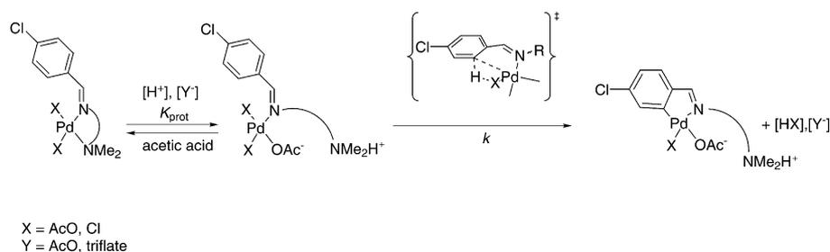
**Scheme 4** Proposed general mechanism for the cyclometallation process studied.
