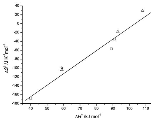
**Fig. 5** Isokinetic relationship for the C–H bond activation on Pd<sup>II</sup> of 4ClC<sub>6</sub>H<sub>4</sub>CHNR containing **1** and **2** ligands in neat acetic acid solvent: Δ corresponds to the acetato derivatives *E*-1AcO and *E*-2AcO, □ to the chloro derivatives, *E*-1Cl and *E*-2Cl, and \* to that of palladium acetate with the equivalent monodentate imine ligand, 4ClC<sub>6</sub>H<sub>4</sub>CHNCH<sub>2</sub>Ph, of ref. 13.
