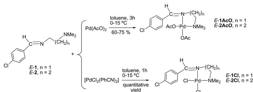
**Scheme 1** Synthesis of type-*E* palladium complexes: **E-1AcO**, **E-1Cl**, **E-2AcO** and **E-2Cl**.
