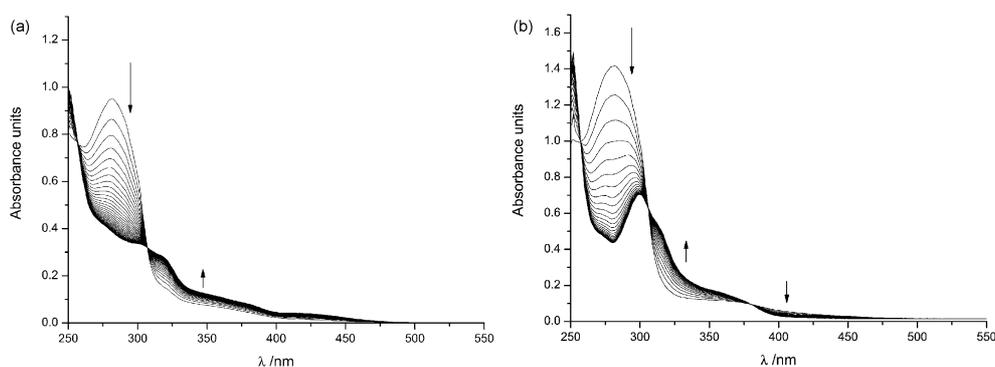
**Fig. 3** (a) UV-Vis spectral changes of the cyclometallation reaction of complex *E-2AcO(M)* in neat acetic acid solution at 40 °C and [Pd] = 1 × 10<sup>−4</sup> M. (b) UV-Vis spectral changes of the cyclometallation reaction of complex *E-2AcO(M)* in triflic acid solutions in acetic acid at 40 °C [HTrif] = 0.012 M and [Pd] = 1 × 10<sup>−4</sup> M.
