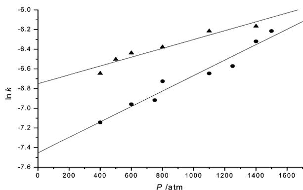
**Fig. 4** Plot for the variation with pressure of the rate constants for the cyclometallation reaction of compounds *E*-1AcO (▲) and *E*-2AcO(M) (●) in acetic acid solution.
