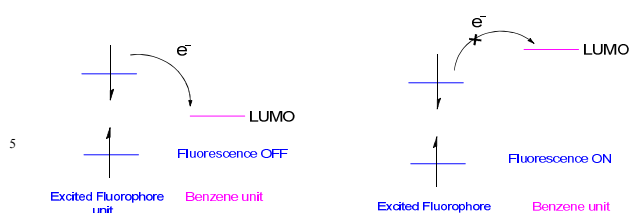
Fig. 3 Schematic diagram of d-PET mechanism
