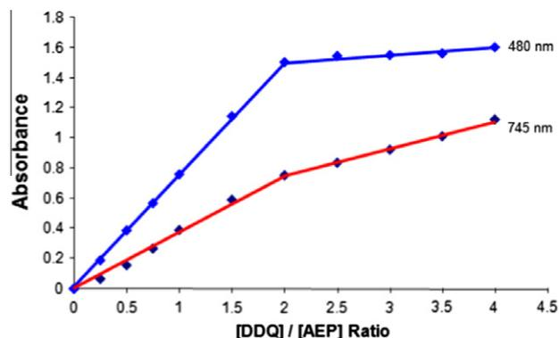
**Fig. 4.** Photometric titration curve for 1-(2-aminoethyl)piperidine (AEP)-DDQ reaction in CHCl<sub>3</sub> measured at 480 nm and 745 nm.
