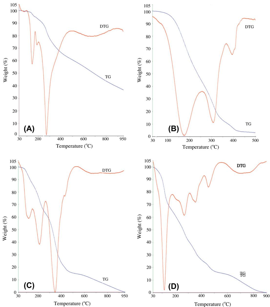
Fig. 14. (A–D) Thermograms of the CT-complexes; (A) [(AEP)(DDQ)<sub>2</sub>], (B) [(AEP)I]<sup>+</sup>I<sub>3</sub><sup>-</sup>, (C) [(AEP)(TCNQ)<sub>2</sub>] and (D) [(AEP)(TBCHD)].
