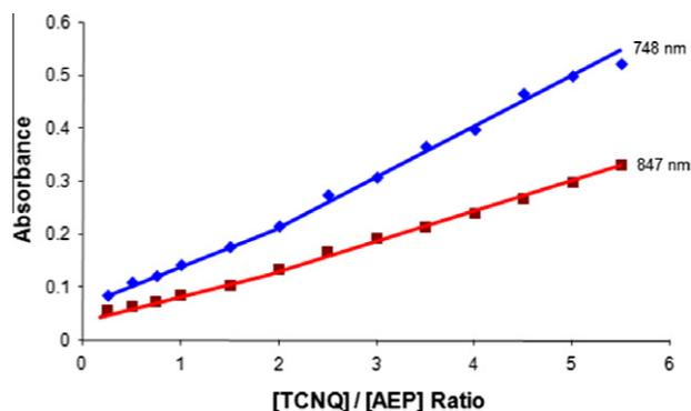
Fig. 6. Photometric titration curve for 1-(2-aminoethyl) piperidine (AEP)-TCNQ reaction in  $\text{CHCl}_3$  measured at 748 nm and 847 nm.
