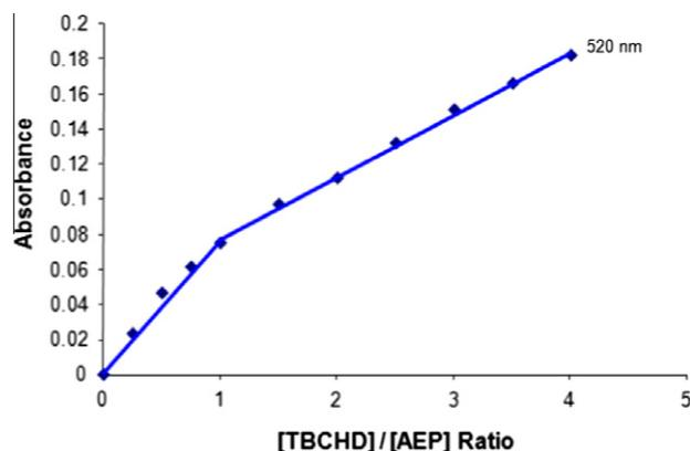
Fig. 8. Photometric titration curve for 1-(2-aminoethyl) piperidine (AEP)-TBCHD reaction in  $\text{CHCl}_3$  measured at 520 nm.
