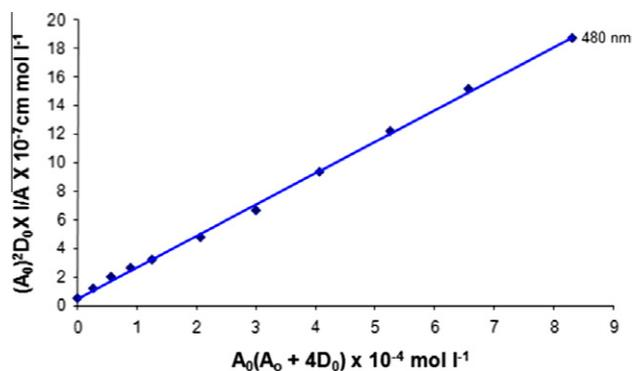
**Fig. 10.** Spectral determination of formation constant and molar extinction coefficient of CT-complex [(AEP)(DDQ)<sub>2</sub>] at 480 nm.
