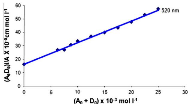
**Fig. 12.** Spectral determination of formation constant and molar extinction coefficient of CT-complex [(AEP)(TBCHD)] at 520 nm.
