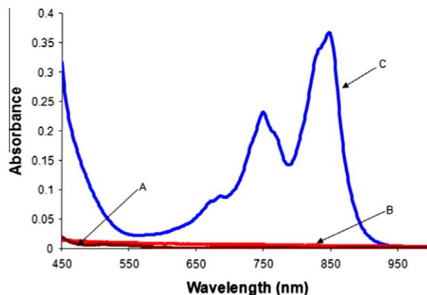
**Fig. 5.** Electronic absorption spectra of 1-(2-aminoethyl)piperidine (AEP)-TCNQ reaction in CHCl<sub>3</sub>. (A) [AEP] = 5 × 10<sup>-3</sup>; (B) [TCNQ] = 1 × 10<sup>-3</sup> M; (C) 1:2 AEP-TCNQ mixture, [AEP] = 5 × 10<sup>-3</sup> M and [TCNQ] = 1 × 10<sup>-3</sup> M.
