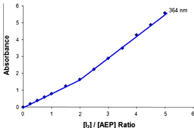
**Fig. 2.** Photometric titration curve for 1-(2-aminoethyl)piperidine (AEP)-iodine reaction in CHCl<sub>3</sub> measured at 364 nm.
