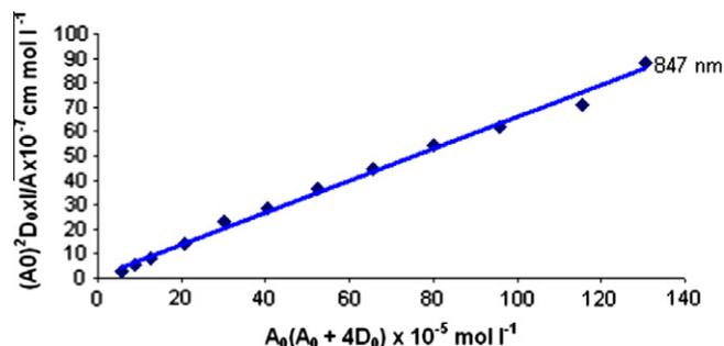
**Fig. 11.** Spectral determination of formation constant and molar extinction coefficient of CT-complex [(AEP)(TCNQ)<sub>2</sub>] at 847 nm.
