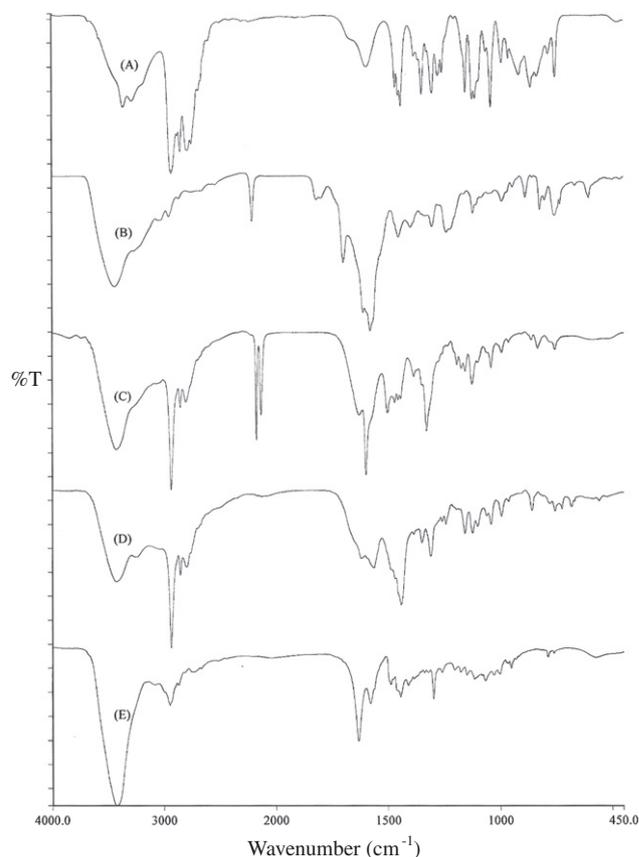
Fig. 13. Infrared absorption spectra of: (A) 1-(2-aminoethyl) piperidine (AEP), (B) [(AEP)(DDQ)<sub>2</sub>], (C) [(AEP)(TCNQ)<sub>2</sub>], (D) [(AEP)(TBCHD)], and (E) [(AEP)I<sup>+</sup>I<sub>3</sub><sup>-</sup>].
