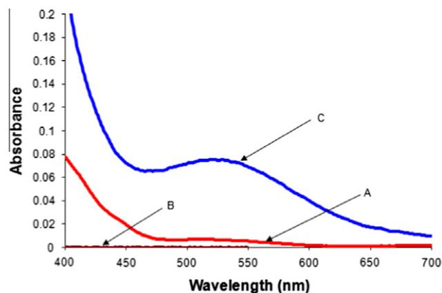
Fig. 7. Electronic absorption spectra of 1-(2-aminoethyl)piperidine (AEP)-TBCHD reaction in  $\text{CHCl}_3$ . (A)  $[\text{AEP}] = 5 \times 10^{-3}$ ; (B)  $[\text{TBCHD}] = 5 \times 10^{-3}$  M; (C): 1:1 AEP-TBCHD mixture,  $[\text{AEP}] = [\text{TBCHD}] = 5 \times 10^{-3}$  M.
