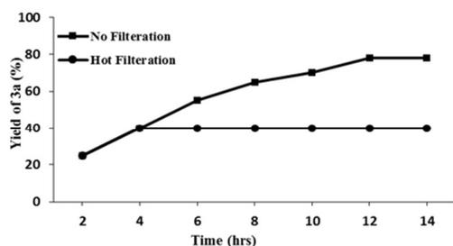
Fig. 3 Hot filtration test for decarboxylative coupling reaction
