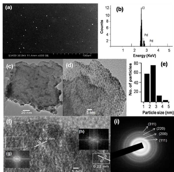
Fig. 1. (a) SEM, (b) EDS, (c) TEM at 20 nm scale, (d) TEM at 5 nm scale, (e) Particle size distribution histogram as calculated from (d), (f) HRTEM image showing lattice fringe spacing, (g), (h) FFT of selected region showing icosahedral and cubic structure of particles, (i) SAED diffraction pattern.
