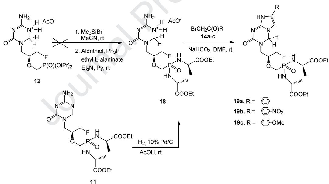
**Scheme 6.** The synthesis of the bis(amidate) prodrug of 5,6-dihydro-FPMP-5azaC (**18**) and its imidazo[1,2-a][1,3,5]triazine analogues (**19a-c**).
