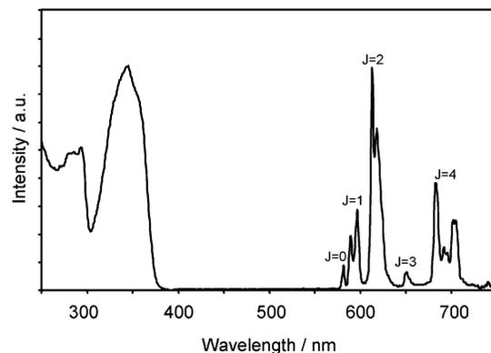
**FIGURE 1.** Corrected excitation (250–450 nm,  $\lambda_{em} = 618$  nm) and emission (550–750 nm,  $\lambda_{ex} = 349$  nm) spectra of the Eu-**6** complex solution (1 × 10<sup>-6</sup> M in borate buffer, pH 8.6). Excitation and emission band-passes 2.5 nm, delay time 0.1 ms, gate time 0.4 ms. The emission bands arise from the <sup>5</sup>D<sub>0</sub> → <sup>7</sup>F<sub>J</sub> transitions; the *J* values are shown on the spectrum.
