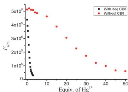
**Fig. 5** Fluorescence response of **SQ2** (5  $\mu\text{M}$ ) in water to  $\text{Hg}^{2+}$  ion in the presence (black squares) and absence (red circles) of 3 equiv. of CB8.
