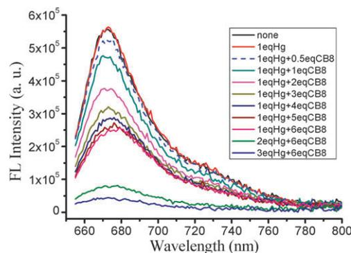
**Fig. 4** Fluorescence spectra of **SQ2** (5  $\mu\text{M}$ ) in water in the presence of different equivalents of **CB8** and  $\text{Hg}^{2+}$ .
