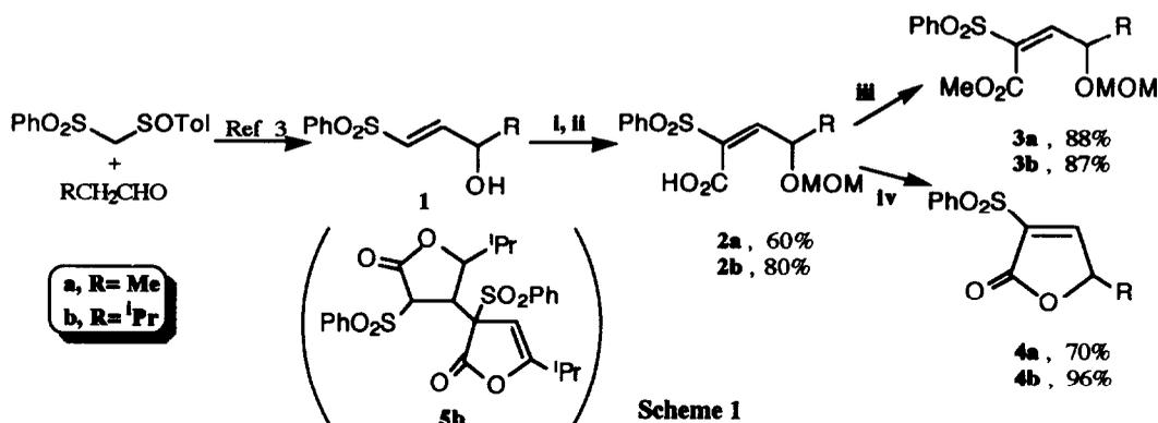
i) CH<sub>2</sub>(OCH<sub>3</sub>)<sub>2</sub>, P<sub>2</sub>O<sub>5</sub>, CHCl<sub>3</sub>, r t, ii) *n*-BuLi or LDA, THF, -78°C, then CO<sub>2</sub>, iii) MeI, NaHCO<sub>3</sub>, DMF, r t, iv) CF<sub>3</sub>SO<sub>3</sub>H, EtOH, r t
