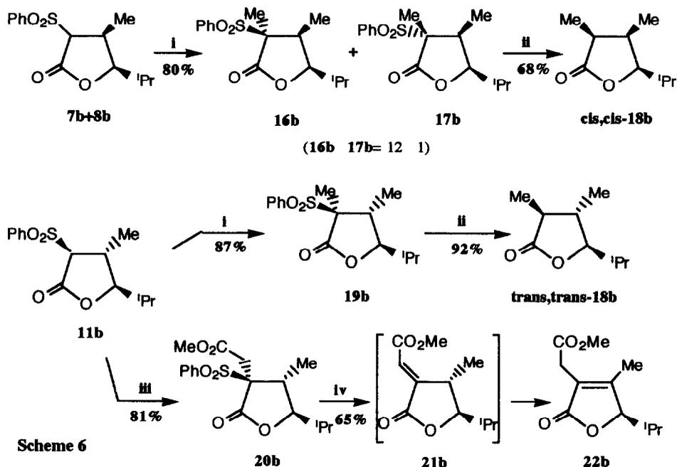
i) MeI, NaH, DMF, 40°C, ii) Na(Hg), Na<sub>2</sub>HPO<sub>4</sub>, MeOH, r t, iii) BrCH<sub>2</sub>CO<sub>2</sub>Me, NaH, DMF, 40°C
