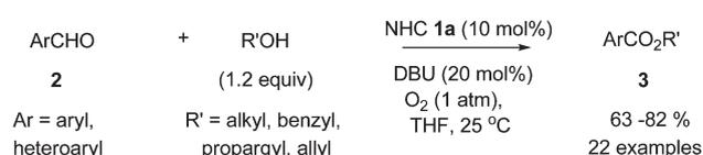
**Scheme 1** NHC catalyzed direct esterification of aromatic aldehydes with alcohols.
