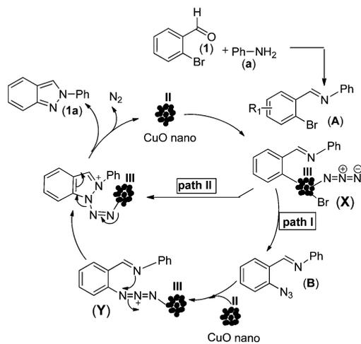
**Scheme 2** Plausible mechanism for the CuO nano catalysed 2*H*-indazoles formation.
