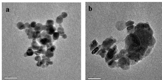
**Fig. 3** TEM images of (a) fresh CuO nano catalyst and (b) CuO nano catalyst after the third cycle.
