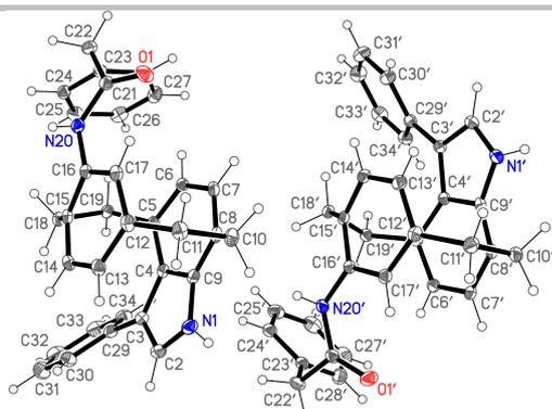
**Figure 10.** Molecular structure of compound **27** (two independent molecules). Ellipsoids represent 30% probability levels.<sup>[23]</sup>
