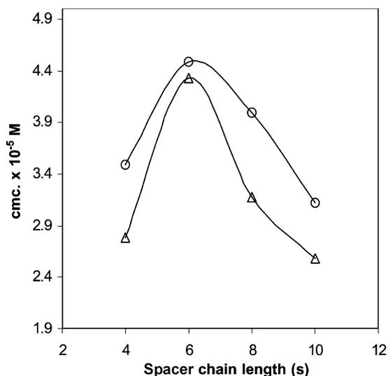
**Fig. 1** Effect of the spacer chain length on the critical micellar concentration of 12-s-12 MEA novel series of bis-cationic surfactants at 30 °C. Variation in the cmc values as a function of spacers chain length, by tensiometry ( $\Delta$ ) and by conductometry ( $\circ$ ).
