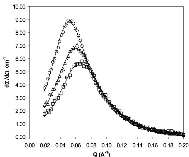
**Fig. 5** Effect of temperatures on SANS distribution for 100 mM 12-4-12 MEA bis-cationic surfactant. The solid line shows the theoretical fits and the symbols are experimentally determined values. 30°C (○), 45°C (△) and 60°C (□).
