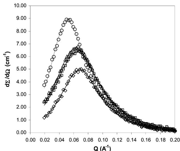
**Fig. 3** Effect of spacer chain length on the SANS distribution for 12-s-12 MEA novel series of bis-cationic surfactants at 100 mM concentrations and 30 °C. The solid line shows the theoretical fits and the symbols are experimentally determined values. s = 4 (○), 6 (△), 8 (□), 10 (◇).
