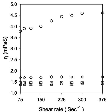
**Fig. 2** Effect of variation of shear rate on absolute viscosity of 12-s-12 MEA novel series of bis-cationic surfactants at 100 mM and 30 °C.  $s = 4$  ( $\circ$ ), 6 ( $\Delta$ ), 8 ( $\square$ ), 10 ( $\diamond$ ).
