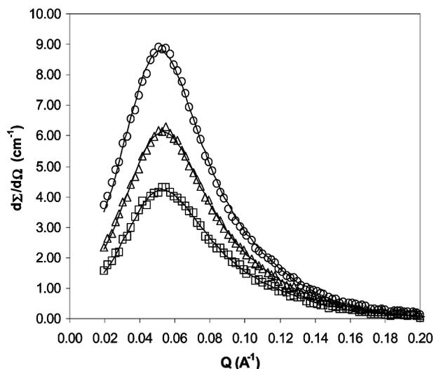
**Fig. 4** Effect of variation of concentration on SANS distribution for 12-4-12 MEA bis-cationic surfactant at 30°C. The solid line shows the theoretical fits and the symbols are experimentally determined values. 100 mM (○), 75 mM (△), 50 mM (□).
