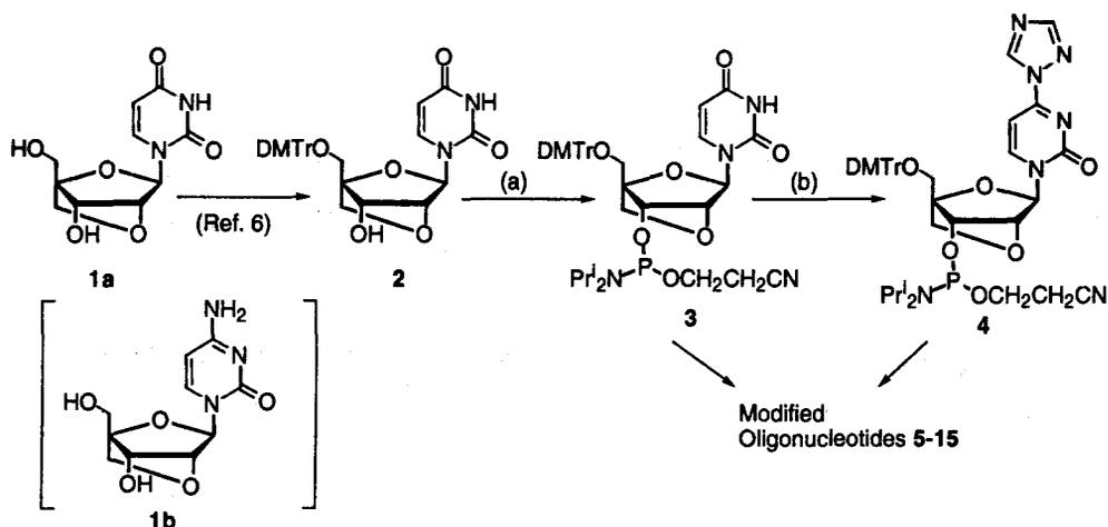
**Scheme 1.** (a) 2-cyanoethyl *N,N,N',N'*-tetraisopropylphosphordiamidite, diisopropylammonium tetrazolide, MeCN-THF (3:1), r.t., 1.5 h, 81%; (b) 1,2,4-triazole, POCl<sub>3</sub>, Et<sub>3</sub>N, MeCN, 0 °C, 4 h, 89%.
