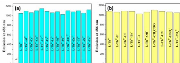
**Fig. 8.** Bar diagram representing performance of optode-10 with 20  $\mu$ M of Th<sup>4+</sup> in the presence of various (a) metal ions (100  $\mu$ M) (b) anions (100  $\mu$ M) in pH 6.5 buffer ( $\lambda_{\text{ex}} = 315$  nm and  $\lambda_{\text{em}} = 486$  nm).
