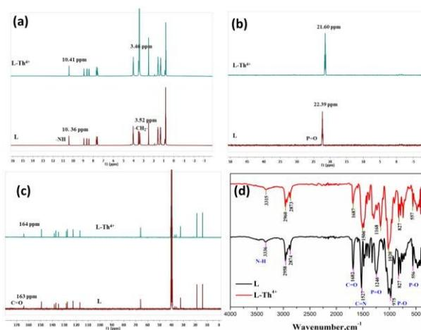
**Fig. 9.** Establishment of binding mechanism of **L** with Th<sup>4+</sup> using (a) <sup>1</sup>H NMR (b) <sup>31</sup>P NMR (c) <sup>13</sup>C NMR for **L** and **L-Th**<sup>4+</sup> complex in DMSO-d<sub>6</sub> (d) FTIR spectra.
