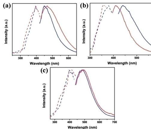
Fig. 5 Excitation (dot lines) and emission (solid lines) spectra of (a) **H<sub>2</sub>BPT** (blue) and **JUC-121** (red), (b) **H<sub>3</sub>IBT** (blue) and **JUC-122** (red), (c) **H<sub>2</sub>TPD** (blue) and **JUC-123** (red).
