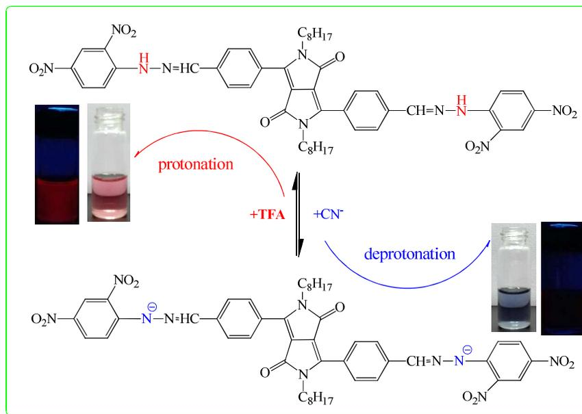
Scheme 2. Proposed interaction mode of receptor 1 with CN<sup>-</sup> and TFA.
