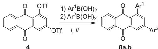
**Scheme 4.** Synthesis of **8a,b**. Reagents and conditions: (i) **4** (1.0 equiv),  $\text{Ar}^1\text{B}(\text{OH})_2$  (1.0 equiv),  $\text{Pd}(\text{PPh}_3)_4$  (3 mol %),  $\text{K}_3\text{PO}_4$  (3.0 equiv), dioxane, 60 °C, 30 h; (ii)  $\text{Ar}^2\text{B}(\text{OH})_2$  (1.2 equiv),  $\text{Pd}(\text{PPh}_3)_4$  (3 mol %), 100 °C, 5 h.
