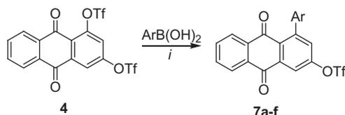
**Scheme 3.** Synthesis of **7**. Reagents and conditions: (i) **4** (1.0 equiv),  $\text{ArB}(\text{OH})_2$  (1.0 equiv),  $\text{Pd}(\text{PPh}_3)_4$  (3 mol %),  $\text{K}_3\text{PO}_4$  (1.5 equiv), dioxane, 60 °C, 30 h.
