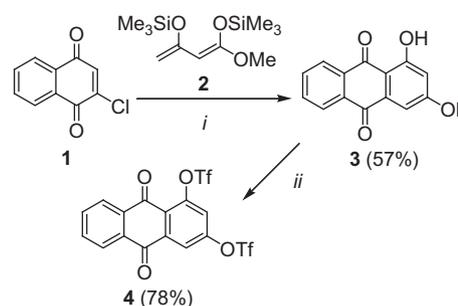
**Scheme 1.** Synthesis of **3** and **4**. Reagents and conditions: (i) (**1**) 1.5 equiv, **2** (1.0 equiv), neat, 20 °C, 12 h; (2) H<sub>2</sub>O; (ii) **3** (1.0 equiv), Tf<sub>2</sub>O (2.4 equiv), pyridine (4.0 equiv), CH<sub>2</sub>Cl<sub>2</sub>, 20 °C, 8 h.
