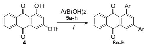
**Scheme 2.** Synthesis of **6a–h**. Reagents and conditions: (i) **4** (1.0 equiv),  $\text{ArB}(\text{OH})_2$  (2.2 equiv),  $\text{Pd}(\text{PPh}_3)_4$  (5 mol %),  $\text{K}_3\text{PO}_4$  (3.0 equiv), dioxane, 100 °C, 7 h.
