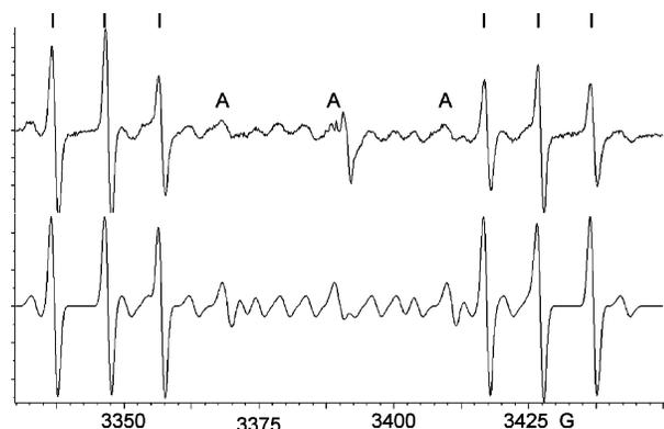
**Figure 1.** Top: EPR spectrum of radicals derived from **1** at 220 K in *tert*-butylbenzene. I = iminyl radical **2**; A = aminoacyl (carbamoyl) radical **3**; other lines are from cyclized radical **4**. Bottom: computer simulation.
